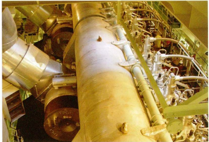
▲ View from above of part of a two-stroke crosshead engine. The diameter of the exhaust gases lead is approximately 3.5 meters!
