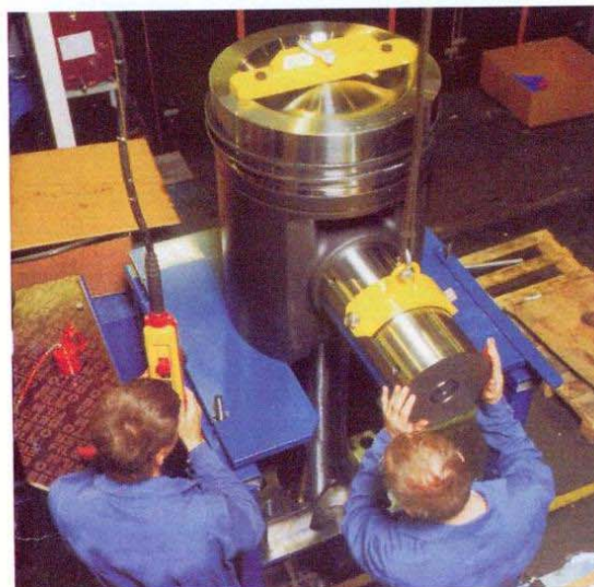
◀ Installing the gudgeon pin in the world's largest four-stroke diesel engine, a Wärtsilä 64 medium-speed diesel engine with a cylinder output of over 2000 kW.
