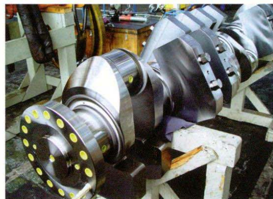
▲ Crank shaft with mounted counter weights for correct balancing.
