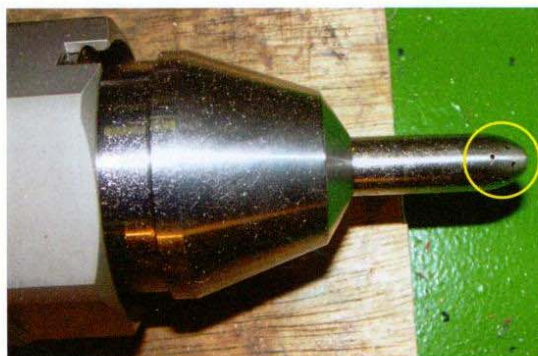
◀ A injector tip of a similar engine with multiple injector apertures.
