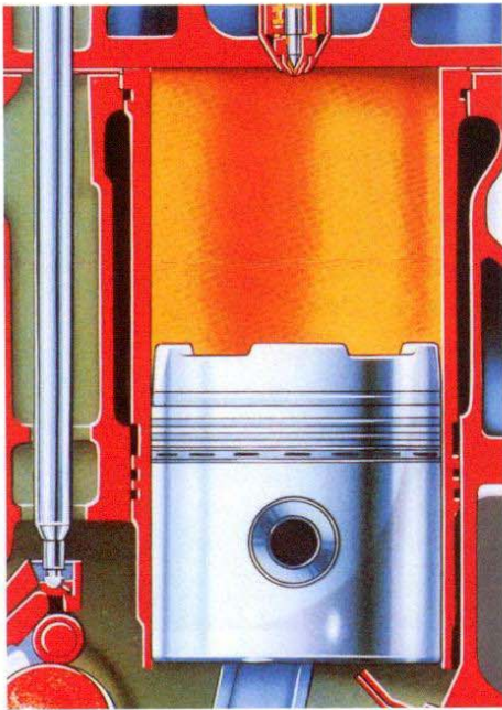
◀ A special aluminium piston for a Cummins-NTA 855 four-stroke high-speed diesel engine.
