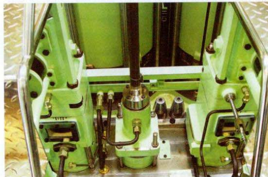
◀ Two high-pressure fuel pumps driven by the camshaft of a MAN-B&W 50 MC crosshead engine.
