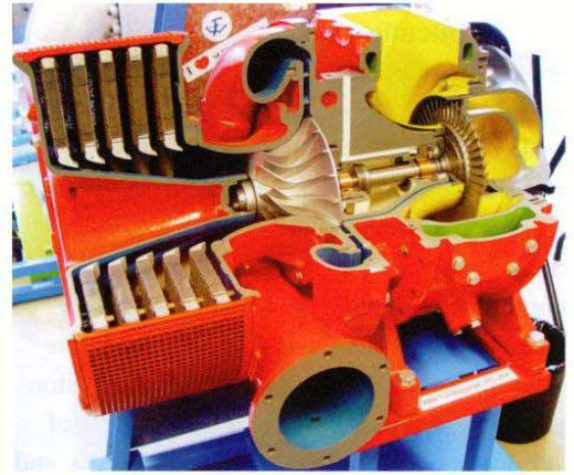
► A cut-away diagram of a turbocharger group.
