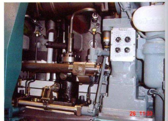
An UG-3 Woodward governor on a medium-speed four-stroke engine of MAN-B&W type 27-38.
