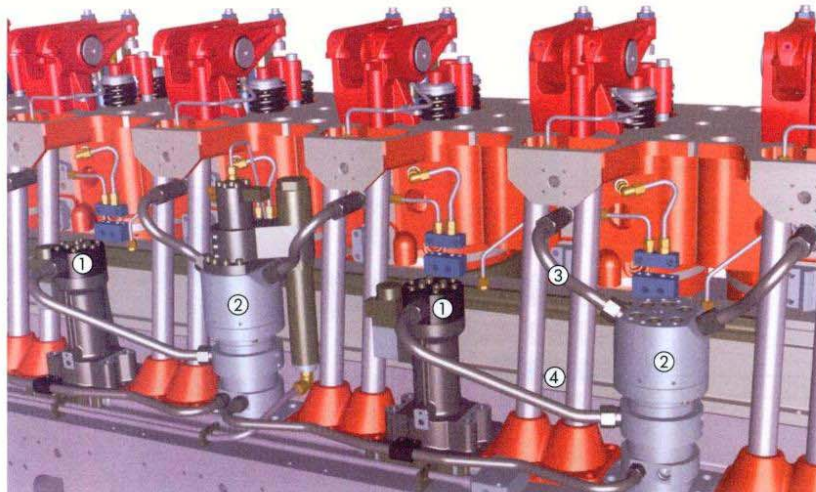
▲ The common rail system for Wärtsilä medium speed four stroke engines, fuel H.F.O.
