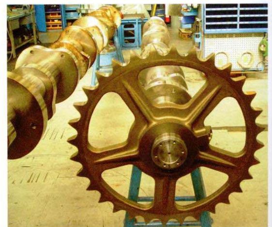
▲ A camshaft for a MAN-B&W K 50 MC two-stroke low-speed crosshead engine.
