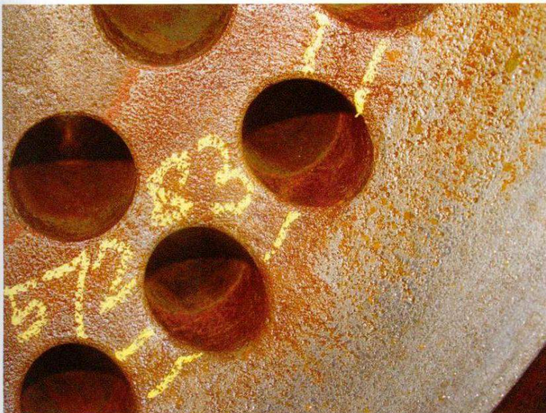
◀ Fissures in the cooling channels of a piston crown in a two-stroke crosshead engine.
