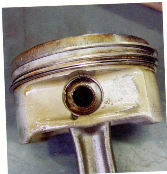
▲ A piston for a small engine with two compression rings and one oil-scraper ring.
