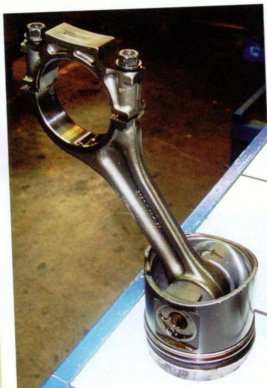
▼ An aluminium piston for an engine category I or II.
