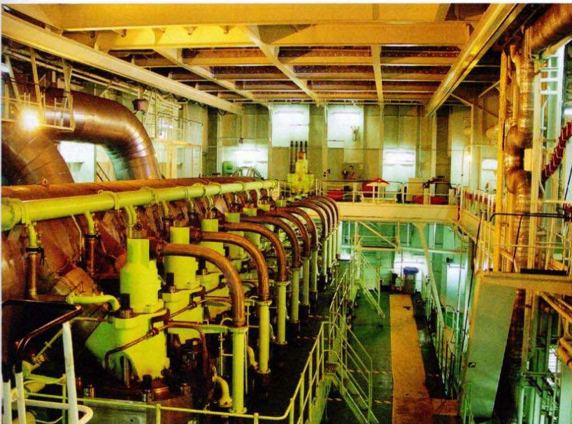
◀ A ten-cylinder two-stroke crosshead engine with the exhaust pipes from every cylinder directly attached to the very spacious central exhaust-gas receiver.
