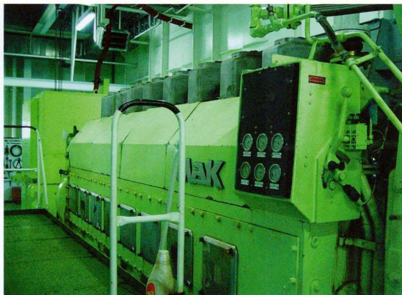
► A Caterpillar-MaK four-stroke diesel engine for the genset in the engine room of a large container ship.
