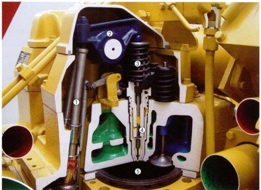
◀ Fuel injectors with mounted the magneto valves.
