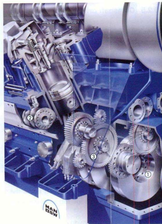
▲ The drive of both camshafts in a V-engine, of RK 280, now MAN-B&W.
