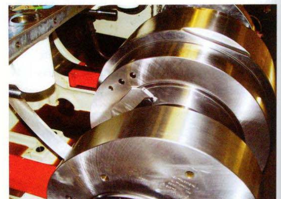
▲ A section of the camshaft for a low-speed two-stroke-crosshead engine, manufacturer Wärtsilä, type RTA 96 C.
