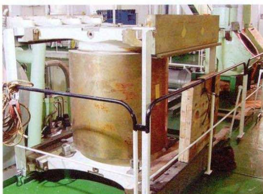
A complete crosshead with crosshead pin and guide shoes.
