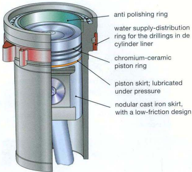
▲ An 'optimum package' of components in the combustion space. Shown the Wärtsilä 32 four-stroke medium-speed diesel engine.
