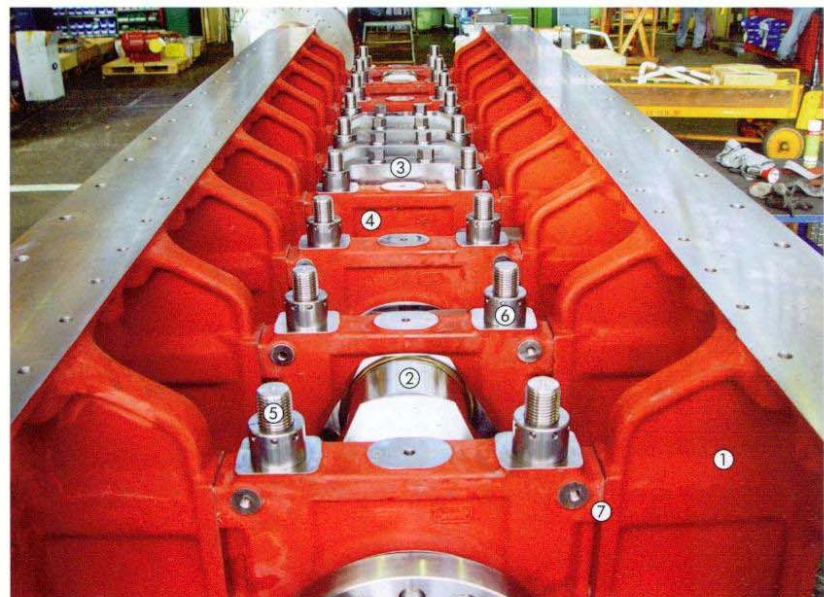
▼ A block in an in-line engine rotated 180° for the mounting of the underslung crankshaft.
