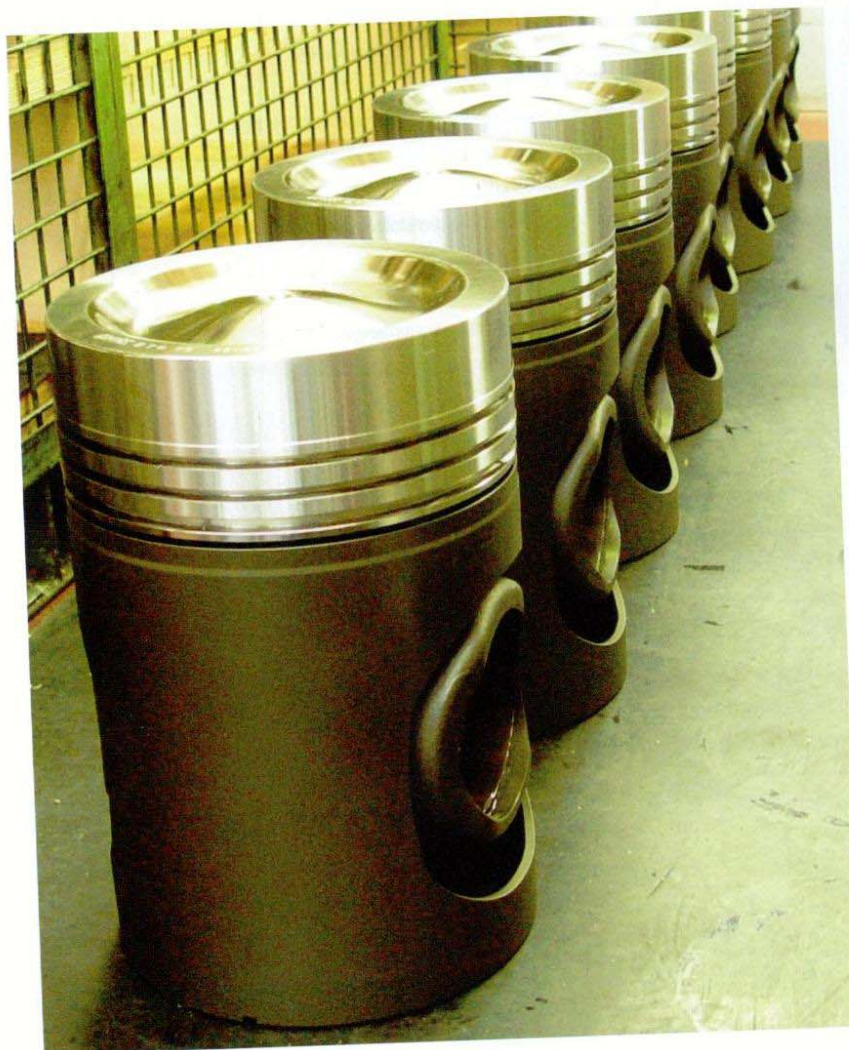
▲ New pistons with a steel crown and a cast iron skirt of Caterpillar-Mak 25 engines.
