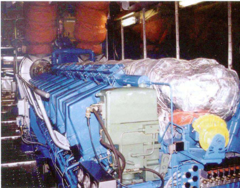
▲ A Woodward PG – governor on a Ruston 20 RK 270 high-speed four-stroke diesel engine running on M.D.O. for a high-speed catamaran of Trasmediterranea.
