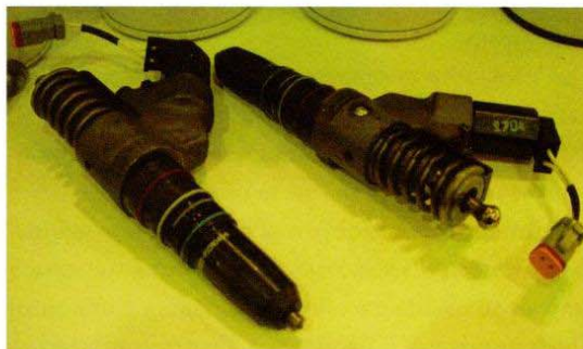
◀ Fuel injectors with mounted the magneto valves.
