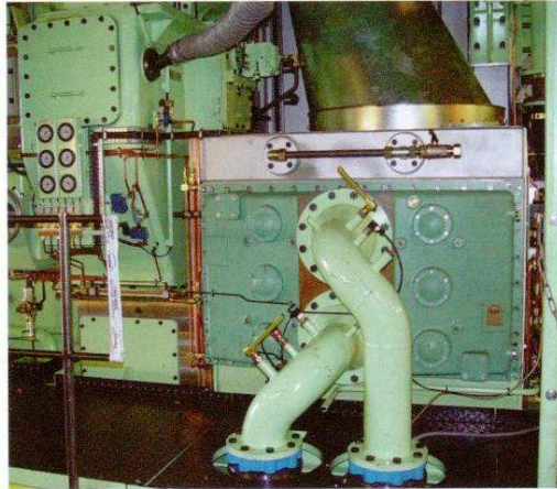
◀ A scavenging air cooler of a two-stroke crosshead engine with the supply and discharge pipes for the L.T. coolant system.
