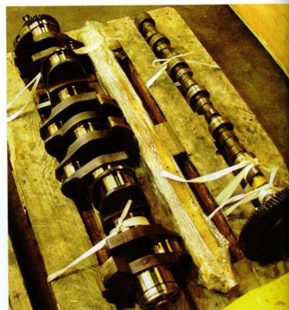
▲ A crankshaft and a camshaft; both forged from one piece for a diesel engine, category II.
